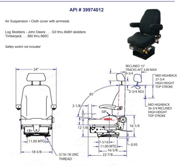
\* OPTIONAL FIELD ADJUSTABLE TRACK MOUNTINGS 12.00" & 13.00". NOTE: Proper length tie-wire must be ordered when modifying track mounting.
