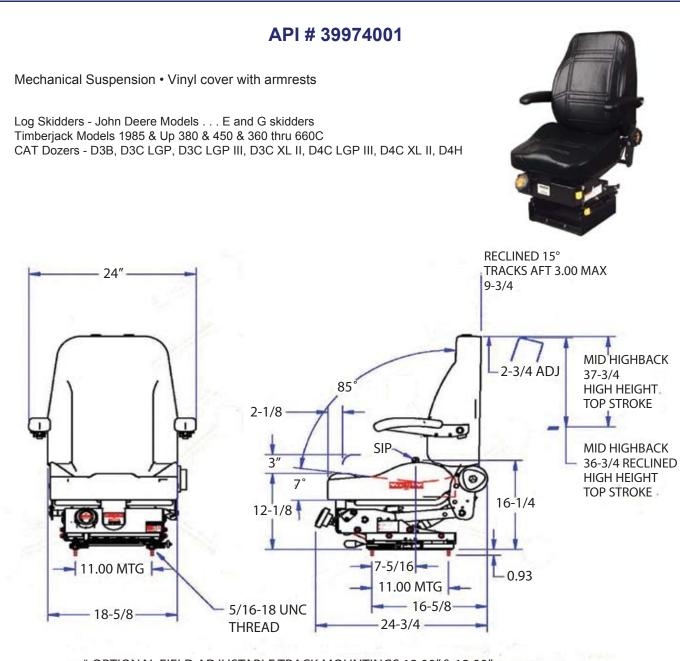
\* OPTIONAL FIELD ADJUSTABLE TRACK MOUNTINGS 12.00" & 13.00". NOTE: Proper length tie-wire must be ordered when modifying track mounting.
