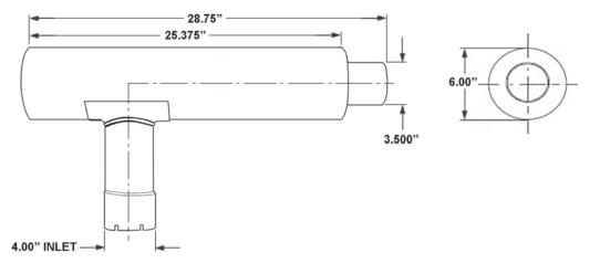
API # 30723000 Prentice Loaders: 210D, 210E, 2180, 410D, 410DX, 410E, 410EX, CRX410D, CRX410E, T180D
