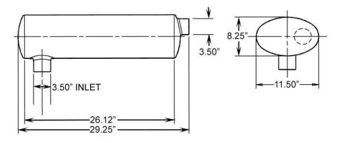
API # 30764000 Timberjack Log Loaders: 330, 430 with Cummins engine
