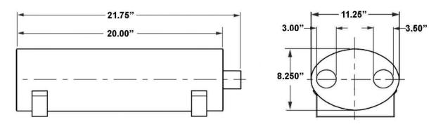
INCLUDES MOUNTING BRACKETS ON EACH END OF THE MUFFLER
